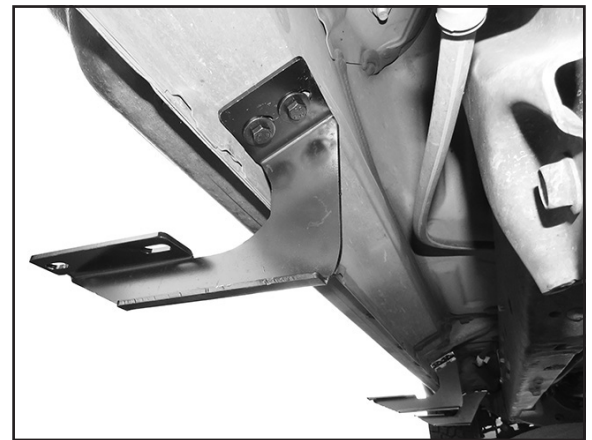
(Figure 7) Driver/left center and rear Mounting Brackets installed.
